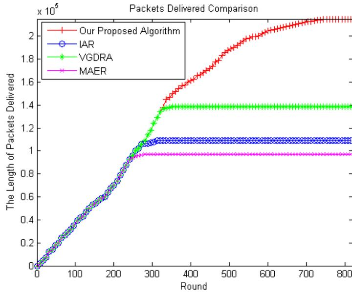
**Fig. 5.** Packets delivered successfully of the four algorithms
